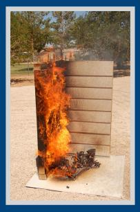
This test photo shows how flames from burning combustible siding can spread upward and expose windows and eaves to flames. The siding that isn't burning is a noncombustible product. Even though it had the same initial fire exposure, the siding did not ignite.
