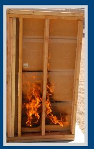
When siding catches fire, the flames can burn into the stud wall cavity at a lap joint, as shown in this test photo. When this occurs, the entire house can be lost to wildfire.
