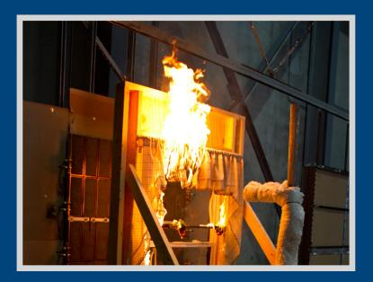
IBHS conducted a test to see whether cotton curtains ignited when exposed to radiant heat that might threaten a window during a wildfire. This test photo shows the curtain burning. However, the curtain only ignited after the glass broke and fell out of the window. This reinforces the advantage of using dual-pane windows, particularly those with tempered glass in the outside panel for the best wildfire protection.
