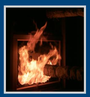
This test photo illustrates how flames can break the glass in a window and penetrate into the interior of a home. Having a dual-pane, tempered glass window offers the best protection because tempered glass does a much better job resisting breakage and even if the outer-pane of glass breaks, the inner pane may remain intact. Keep all windows closed during wildfires – the most vulnerable window during a wildfire is one that is left open.
